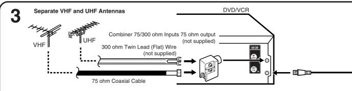
**Note:** If both VHF and UHF antennas have 300 ohm twin lead (flat) wires, use a combiner having two 300 ohm inputs and one 75 ohm output.
